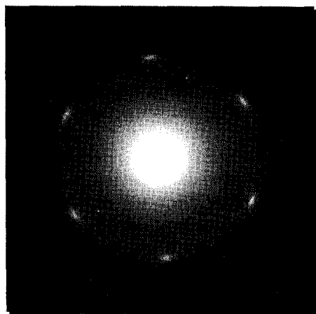
Fig. 9. ED pattern of the C_{60} monolayer prepared by the multi-step creep method.
